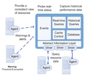
Figure 6: The GridRM Architecture
