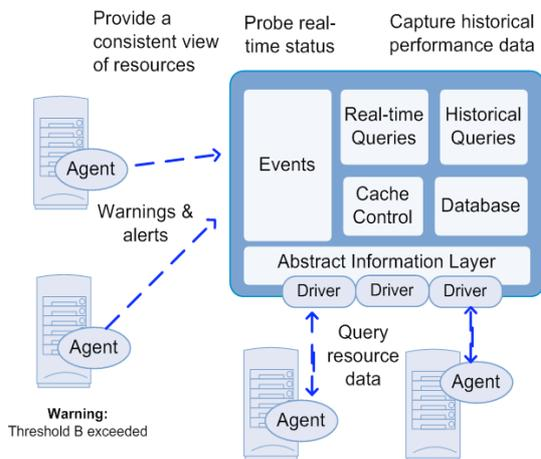
Figure 6: The GridRM Architecture
