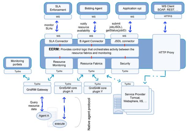
Figure 7: The SORMA EERM Architecture
